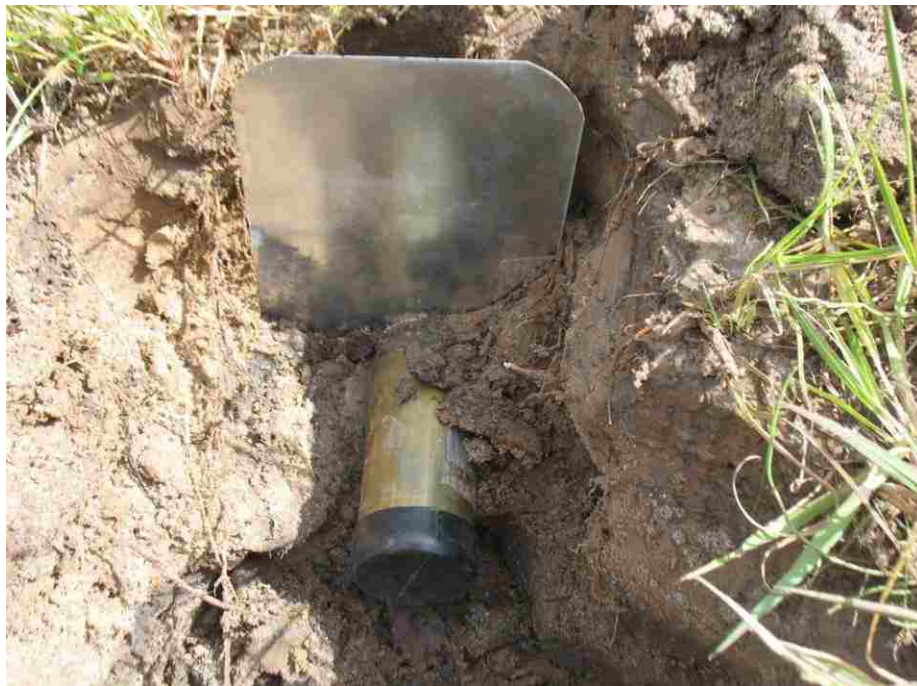
Figure 20. A core sample taken from layer 2 composed primarily of sand
