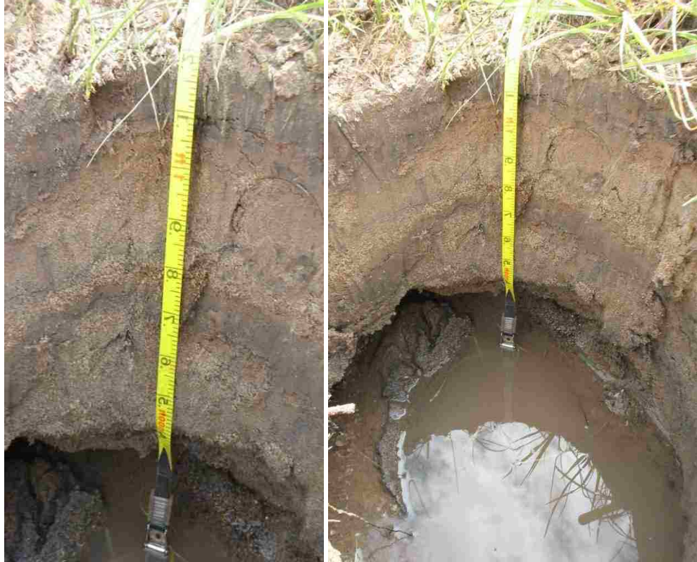
Figure 19. The lithology of site 1 with alternating layers of fine and coarse sediments
