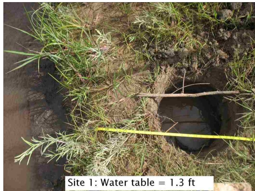
Figure 18. The exposed hole that was used to obtain the samples from site 1
