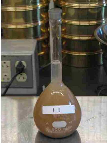
Figure 31. Sample 1, layer 1 specific gravity test with the sieves for the particle size distribution in the back
